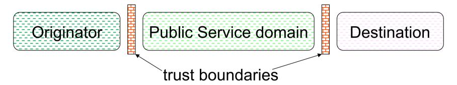
Originator and Destination are customer networks (stub networks in terms of IP routing)
